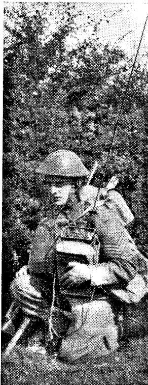
This small infantry pack set (No. 38) employs a throat microphone and is so arranged that it does not interfere with the wearer's fighting efficiency.
